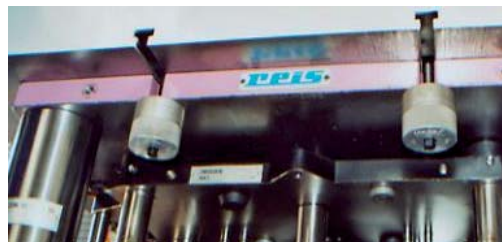
MCA- power clamping nut for clamping of upper and lower die in a hydraulic press
