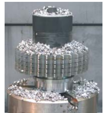
Power clamping nut MDA for clamping of chain wheels during milling
