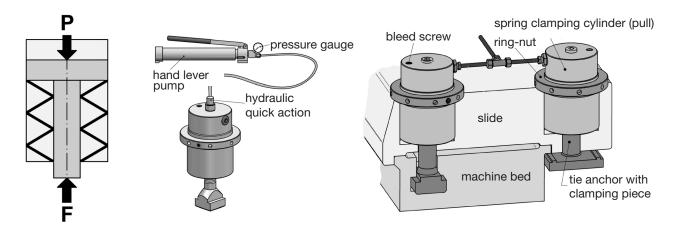
Note: If automatic clamping operation is not required, the temporary, manual hydraulic connection to a manually operated piston pump with a pressure gauge provides a cost effective alternative (see fig. at left).
