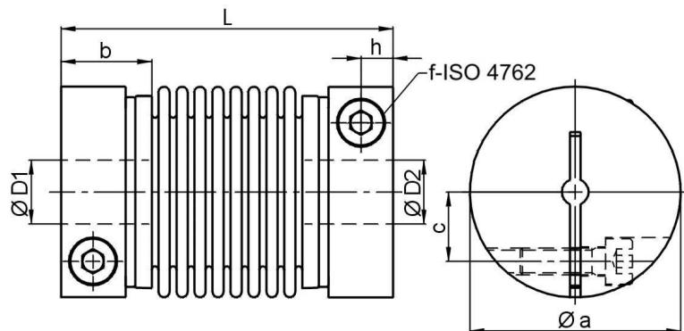
Dimensions [mm]: length dimensions according to DIN ISO 2768 cH
