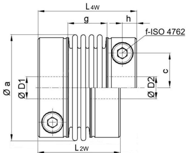
**notes:** connection between bellows and hub by plasma welding. Three standard versions with 6-corrugation bellows 6W, 4-corrugation bellows 4W or 2-corrugation bellows 2W. Size 1.5 with 5-corrugated metal bellows.
