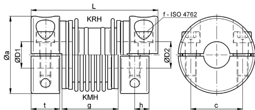
Dimensions [mm]: length dimensions according to DIN ISO 2768 cH
