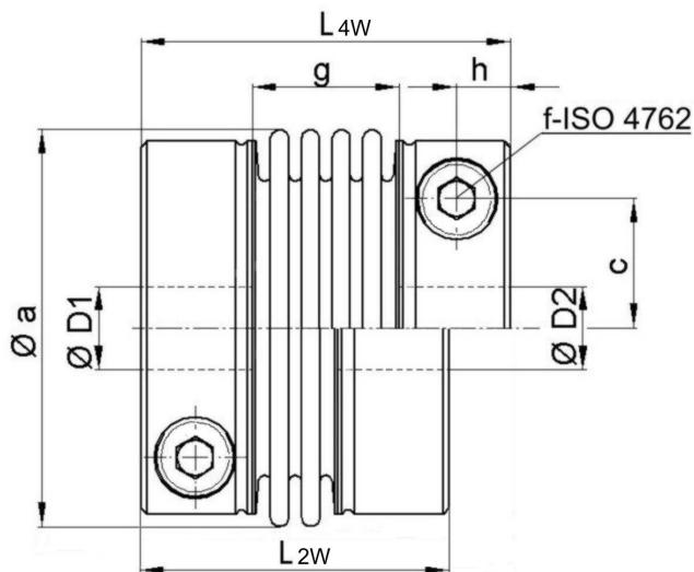
**notes:** connection between bellows and hub by plasma welding. Three standard versions with 2-corrugated metal bellows 2W, 4-corrugated metal bellows 4W or 6-corrugated metal bellows 6W.
