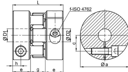
Dimensions [mm]: length dimensions according to DIN ISO 2768 cH
