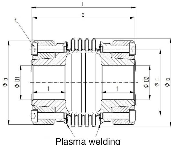
Dimensions [mm]: length dimensions according to DIN ISO 2768 cH
