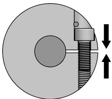
The clamping hub is backlash-free and force-fitted with the shaft.
