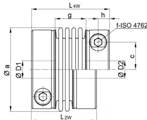
**note:** connection between bellows and hub by plasma welding
