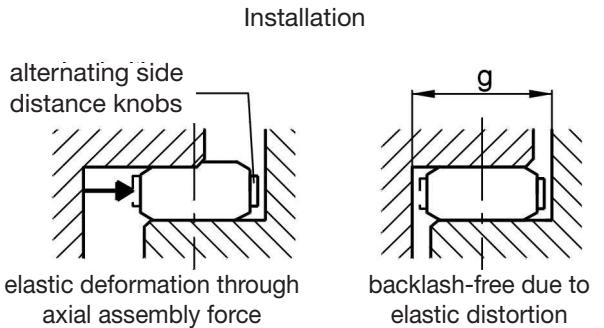
**tolerable seat clearance shaft / hub:** Series ESM-A: max 0,02 mm
