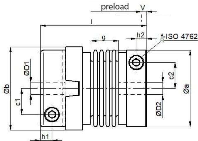
Dimensions [mm]: length dimensions according to DIN ISO 2768 cH
