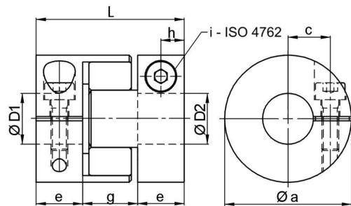
Dimensions [mm]: length dimensions according to DIN ISO 2768 cH
