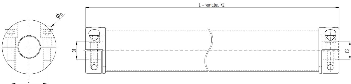
material: hub: high-tensile aluminum intermediate pipe: CFK
