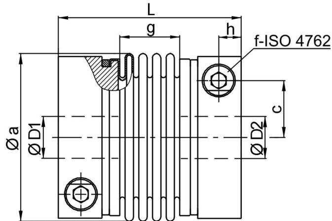
Dimensions [mm]: length dimensions according to DIN ISO 2768 cH
