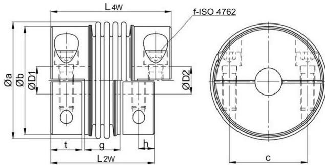
**note:** Standard versions with 6-corrugated metal bellows 6W, 4-corrugated metal bellows 4W or with 2-corrugated metal bellows 2W -> see values in brackets. Connection of bellows and hubs by micro-plasma welding process.
