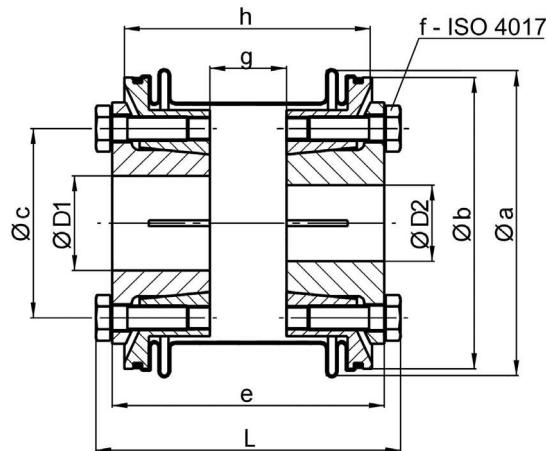
Dimensions [mm]: length dimensions according to DIN ISO 2768 cH
