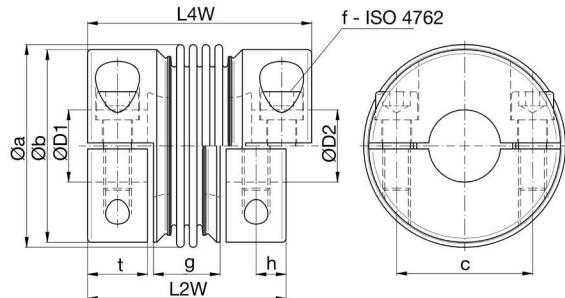
note: connection between bellows and hub by plasma welding
