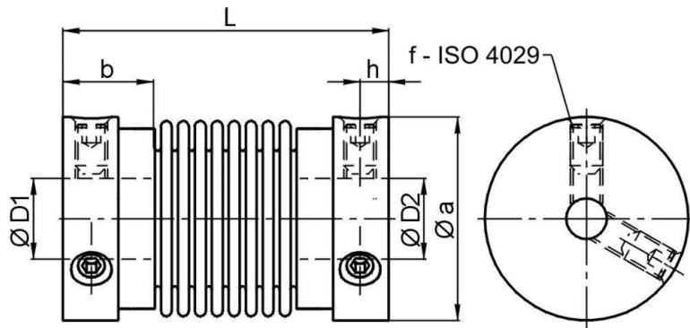
Dimensions [mm]: length dimensions according to DIN ISO 2768 cH
