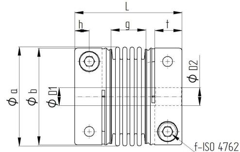
**note:** Connection of bellows and hubs by micro-plasma welding process.
